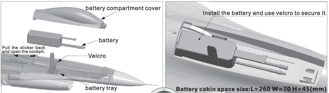
Before connecting the battery to the ESC, please switch on the transmitter and make sure the throttle is in the lowest position. Use a the kill switch if you have one assigned.
